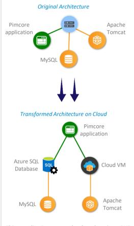
This application was developed using PHP platform as a single-tier application and hosted on Apache HTTP web server with MySQL as database server.
