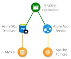
This application was developed using Java platform as a single-tier application and hosted on Apache Tomcat web server with MySQL as database server.
